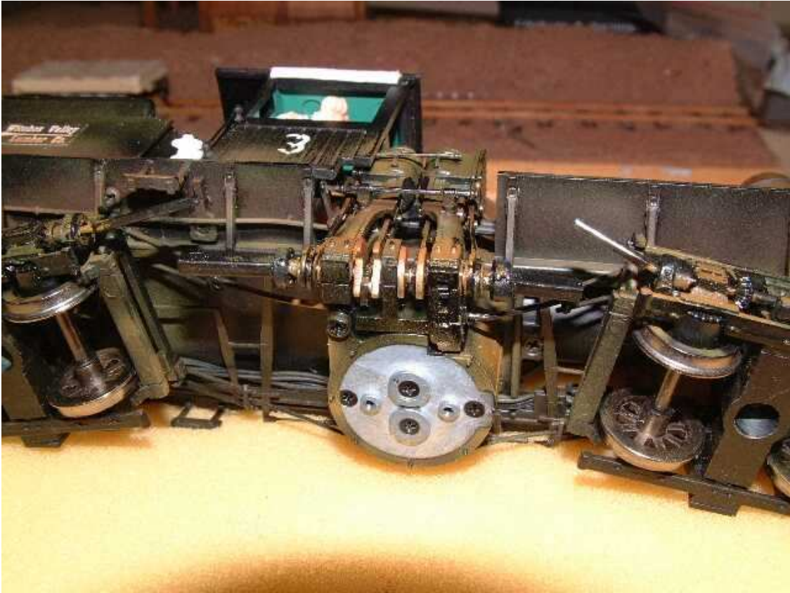
Step# 3 Open the U-joints by turning the trucks.
