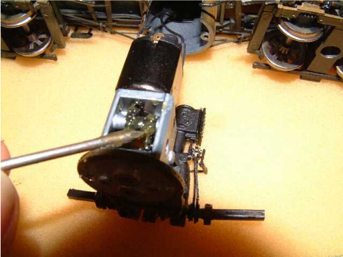
Step # 9 Use grease and a toothpick to lubricate the gears.
