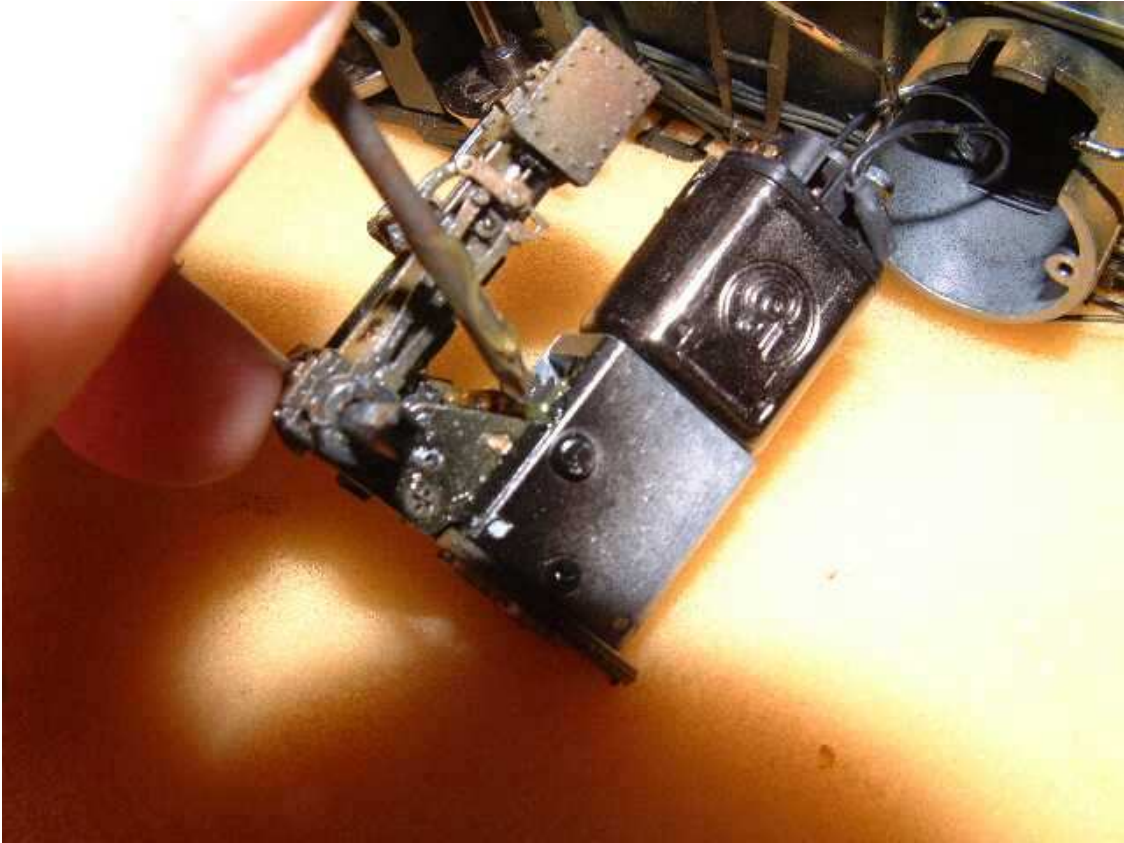
Step # 11 Add some grease to the gears going from the gearbox to the cylinders
