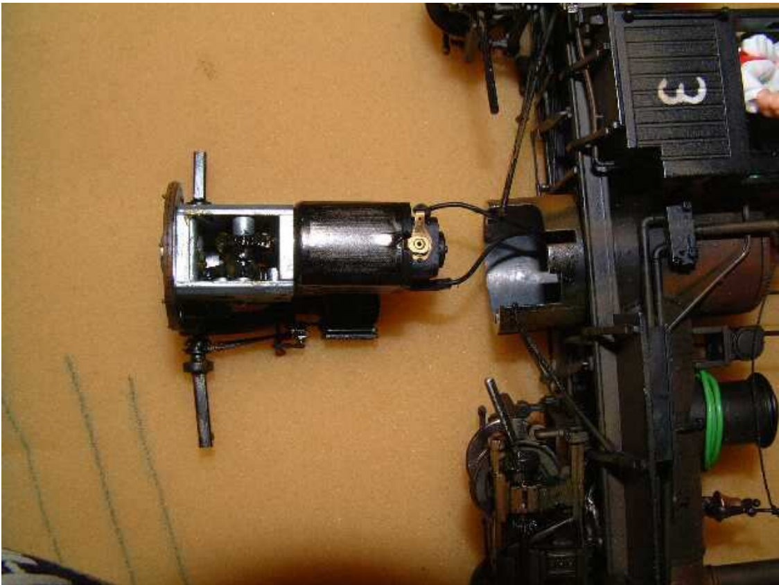
Step # 10 Use a drop of oil to lubricate the bearings at the motor.
